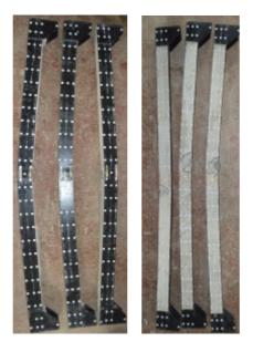
Figure 9 – The destruction of experimental steel-concrete samples with sheet reinforcement of the series SB-PD-24-1..3 and SB-PN-24-1..3 nature
