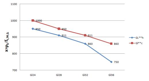
Figure 5 – The illustration of X parameter for glued laminated timber
