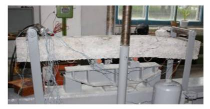
Figure 9 – Investigation of beam 1B – FC – 1 on flexure
