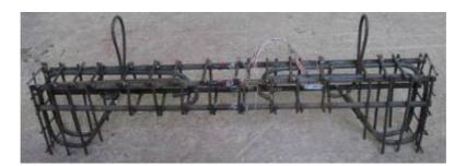
Figure 4 – Spatial reinforcing cage for reinforced concrete columns
