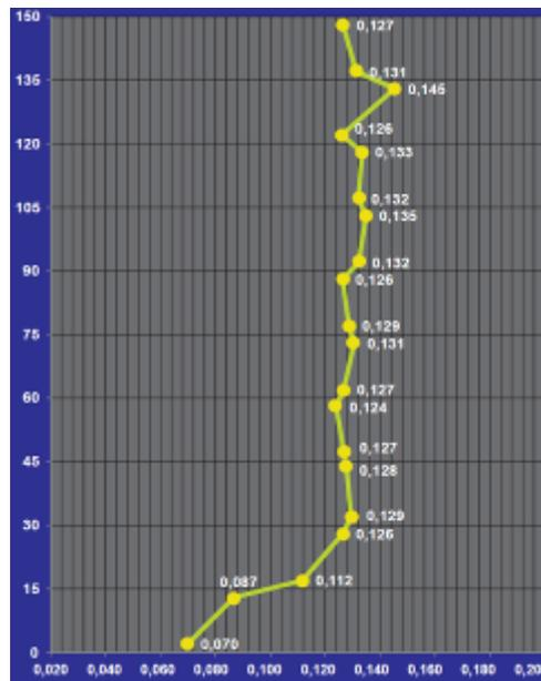
**Figure 2 – Soil moisture plot changes depending on pipe height – moisture plot changes of compacted light silt loam, compacted at moisture corresponding to stabilized moisture value  $w = w_k = 0,130$ , to soil skeleton density  $\rho_d = 1,60 \text{ g/cm}^3$  and pipe height of 150 cm,**
